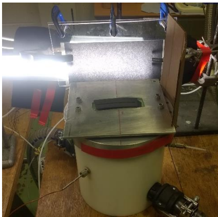
PSN flow testing rig (left) and BOS of flow field (right).
