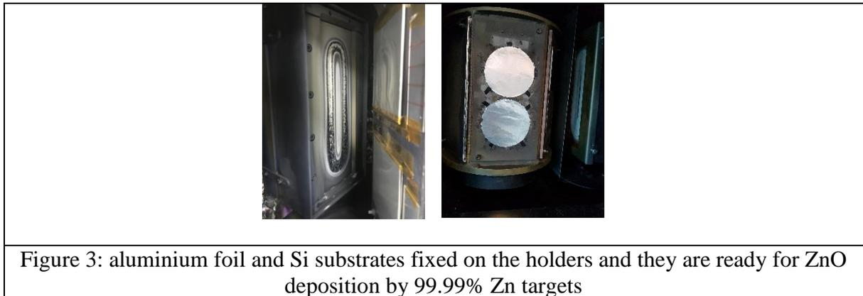
Figure 3: aluminium foil and Si substrates fixed on the holders and they are ready for ZnO deposition by 99.99% Zn targets
