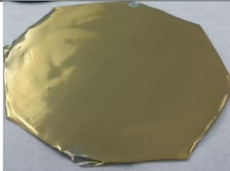
Figure 4: ZnO deposited on Al film
