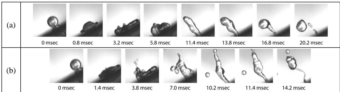
Figure 1: Droplet impact on a SAW device with inclination angle of 30 degree. The applied power is (a) 5 w (b) 15 w. For this experiment SAW travels upward.
