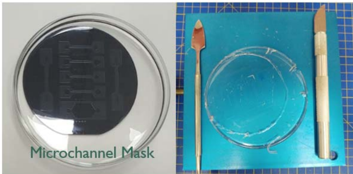
Figure 1 Microchannel mask and uncut PDMS microchannels.
