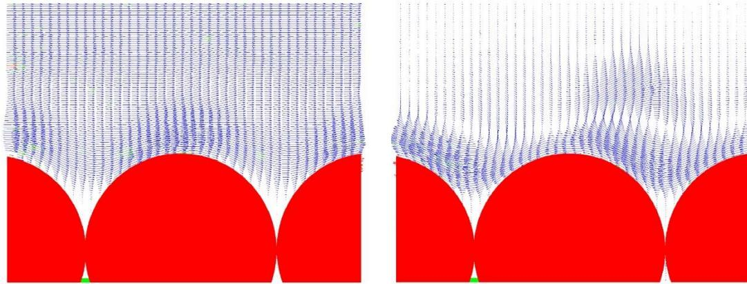
**Figure 2:** Example velocity vector maps. Left: velocity field at maximum free-stream velocity; right shows the velocity field at free-stream flow reversal. The free-stream velocity has a period of 1.65s and amplitude of 0.06 m. The masked glass marbles have a diameter of 10mm. PIV sampling rate 500 Hz.
