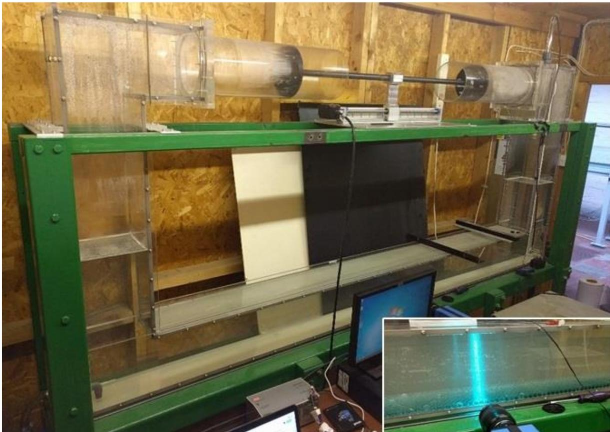
**Figure 1:** Dundee's Oscillatory Flow Tunnel facility, the insert shows the high-speed camera and laser sheet over a glass marble-covered bed.
