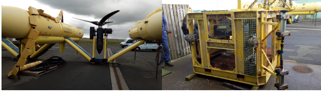
Figure 2 Tidal energy devices: tidal turbine (left) and testing sensor platform (right)
