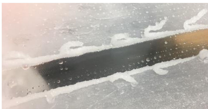
Fig 3.14: WSP detaching from the ridge
