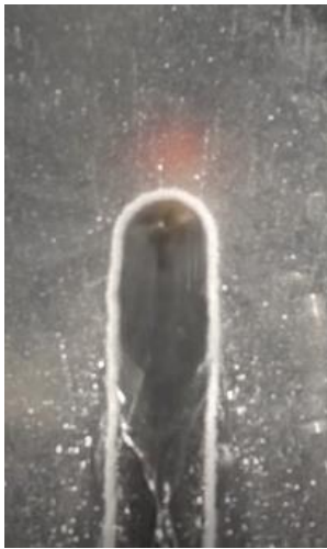
Fig. 3.10: Clean area for 0.2mm film, 2.9\text{cm s}^{-1} moving jet
