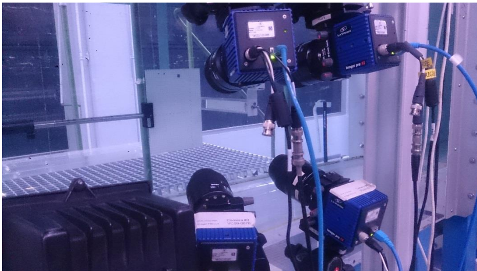
Figure 1. Calibration process for tomographic PIV. Cameras (foreground) with a calibration plate held in the channel (white rectangle). Wakes are generated by the square bar to the right of the calibration plate.
