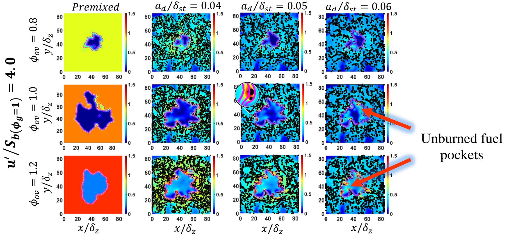
Distribution of  $Y_F/Y_{st}$  (magenta lines show  $c = 0.1, 0.5, 0.9$  contours from outer to inner periphery) on the central  $x$ - $y$  mid-plane for turbulent flames with  $\phi_{ov} = 0.8, 1.0$  and  $1.2$ . All figures correspond to  $t = 2.52\alpha_{T0}/S_b^2(\phi_g=1)$
