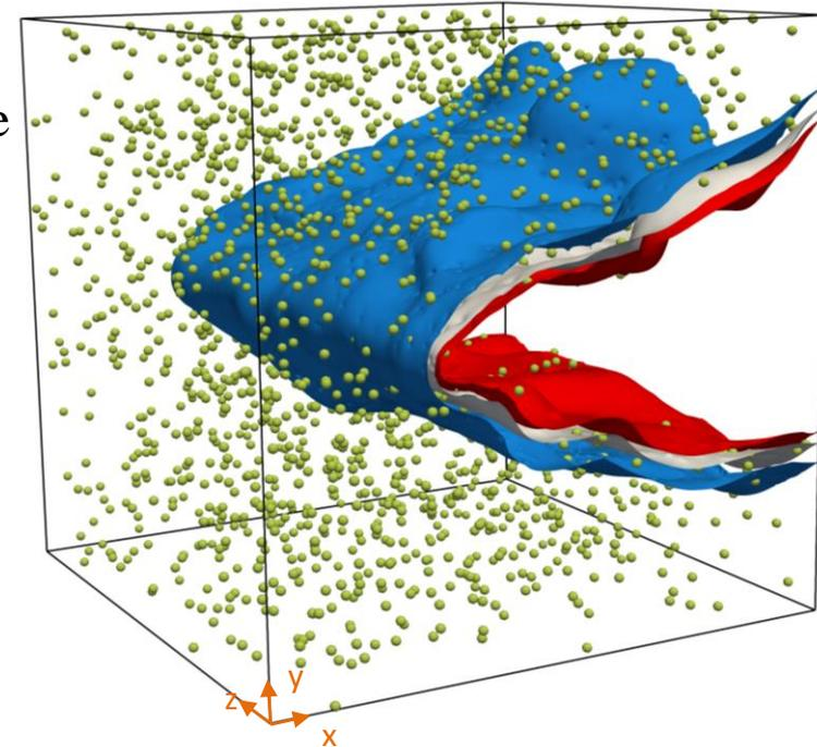
Reaction progress variable isosurfaces at  $c = 0.1, 0.5$  and  $0.9$  for  $a_d/\delta_{th} = 0.06$  initial droplet diameter, at  $t = 1.5t_{flow}$ .
