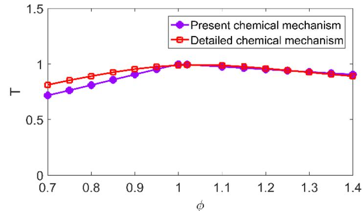
Variation of the (a) normalised laminar burning velocity  $S_b(\phi_g)/\{S_b(\phi_g)\}_{max}$  and (b) normalised adiabatic flame temperature  $T_{b(\phi_g)} = (T_{ad}(\phi_g) - T_0)/(T_{ad}(\phi_{g=1}) - T_0)$  with equivalence ratio  $\phi_g$  for n-heptane obtained from modified single step chemistry (Tarrazo *et al.*, 2006), detailed chemical mechanism (Chaos *et al.*, 2007) and experimental (Kumar *et al.*, 2007) data.
