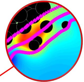
Distribution of  $Y_F/Y_{St}$  (magenta lines show  $c = 0.1, 0.5, 0.9$  contours from outer to inner periphery) on the central  $x$ - $y$  mid-plane for laminar flames with  $\phi_{ov} = 0.8, 1.0$  and  $1.2$ . All figures correspond to  $t = 2.52\alpha_{T0}/S_b^2(\phi_g=1)$
