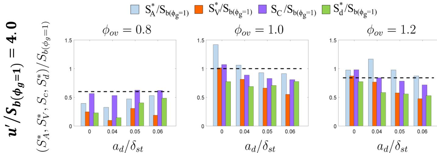
Mean values of  $S_C/S_b(\phi_g=1)$  and  $S_d^*/S_b(\phi_g=1)$  on  $c = 0.8$  isosurface along with alternative flame speeds  $S_A^*/S_b(\phi_g=1)$  and  $S_V^*/S_b(\phi_g=1)$ . The value of  $S_b(\phi_g=\phi_{ov})/S_b(\phi_g=1)$  is shown by the horizontal black dashed line.
