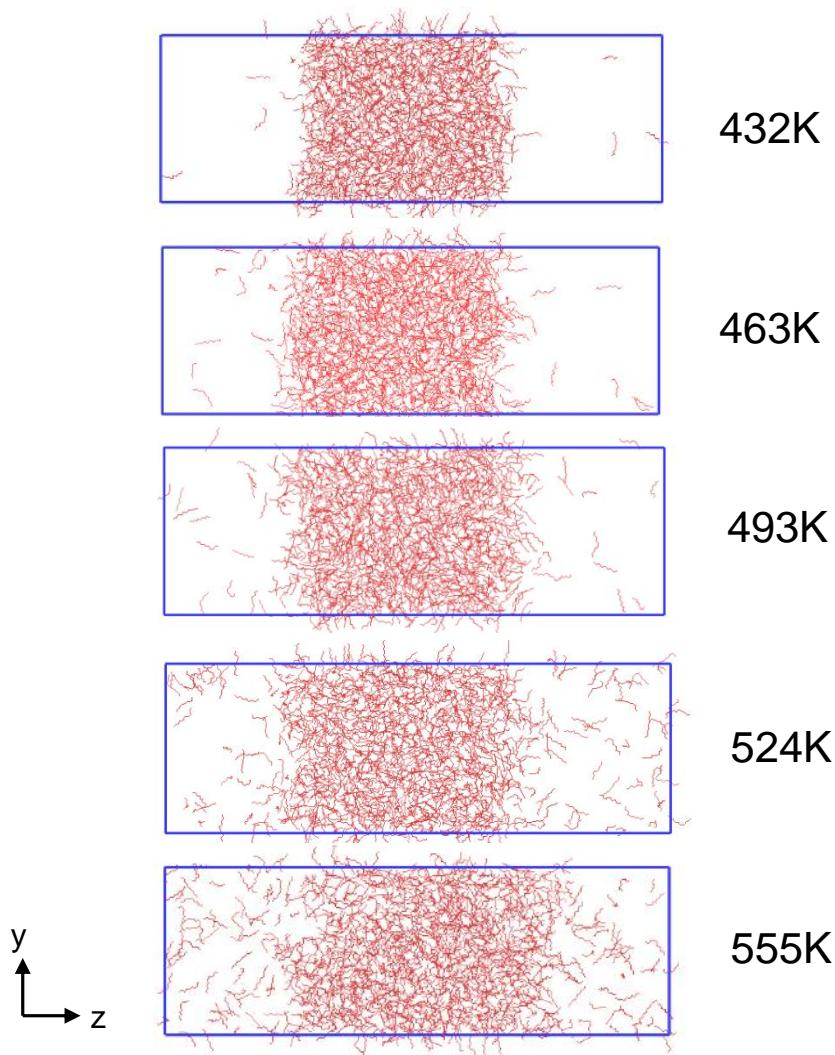
*Evaporation of n-decane at different temperatures*
