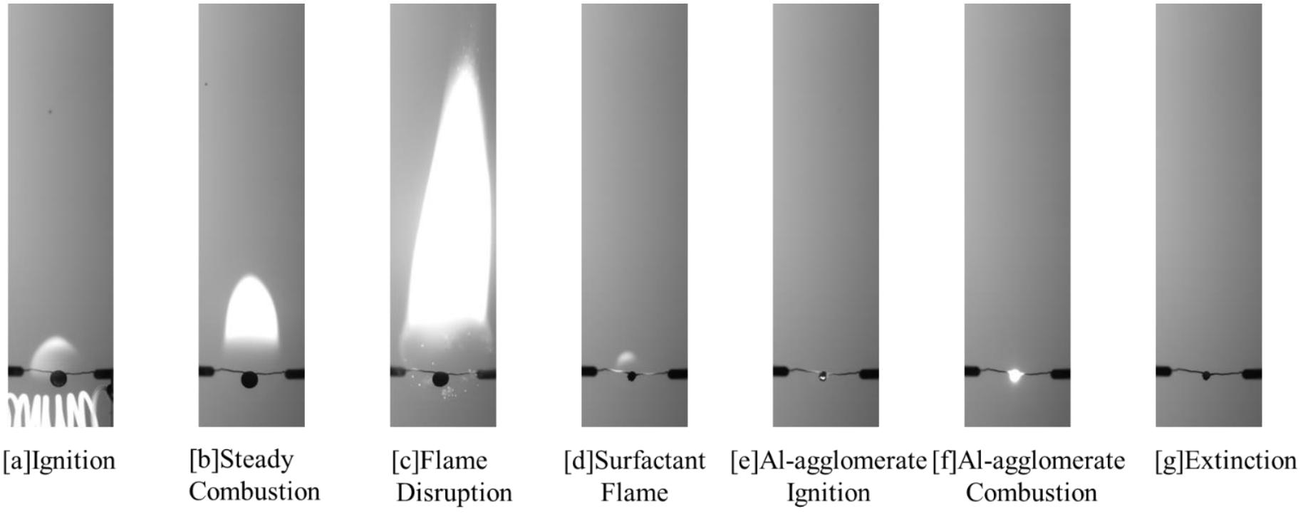
*A burning sequence of RP-3/nano-Al droplet at 0.5bar*
