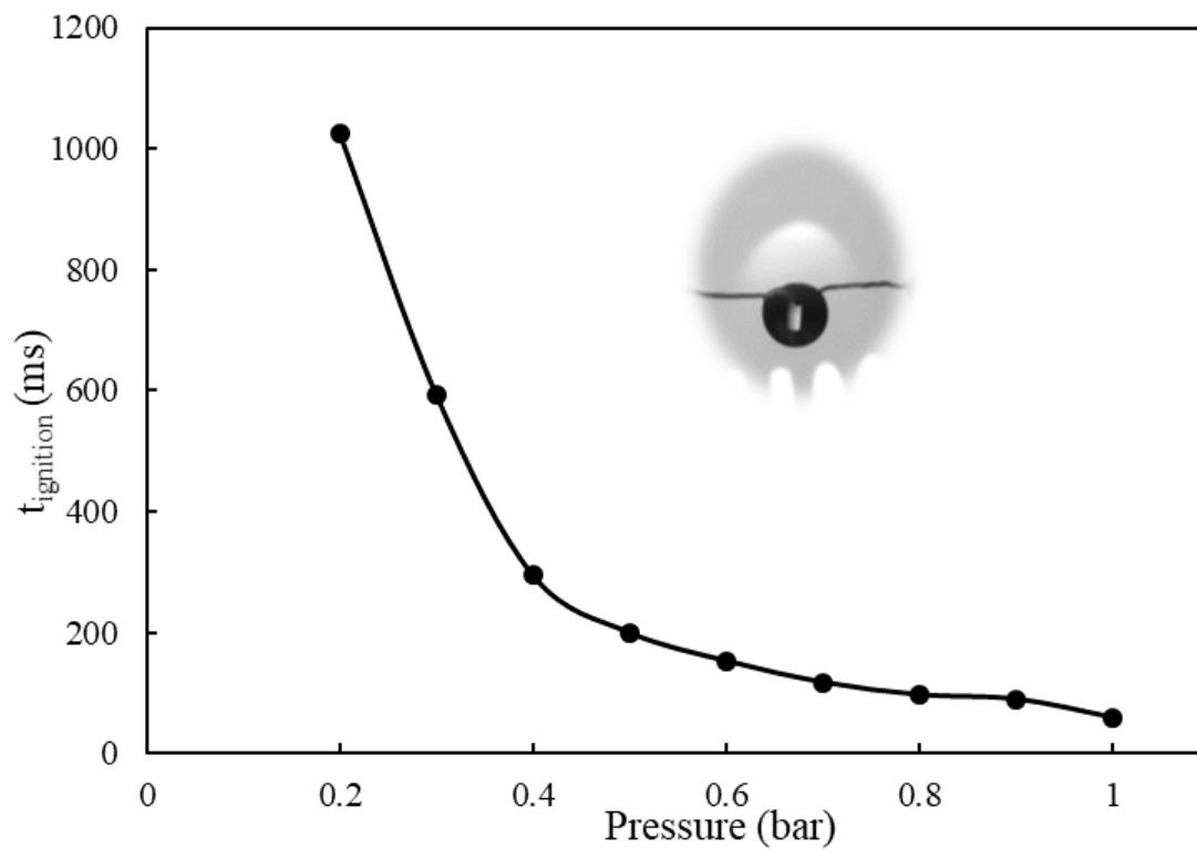
*Ignition delay time at different pressures for RP-3 kerosene*
