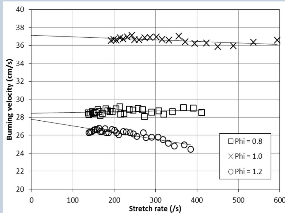
Stretch rate against burning velocity for biogas mixtures of 80% methane at  $T_0 = 450$  K and  $P_0 = 4$  bar.
