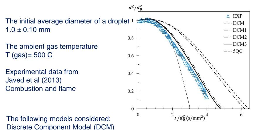
DCM as above and the contribution of supporting fibre (plots DCM1); DCM as above accounting for natural convection (plots DCM2); DCM as above accounting for natural convection and supporting fibre (plots DCM3); 5 Quasi components, Multi-Dimensional Quasi-Discrete Model (5QC)
