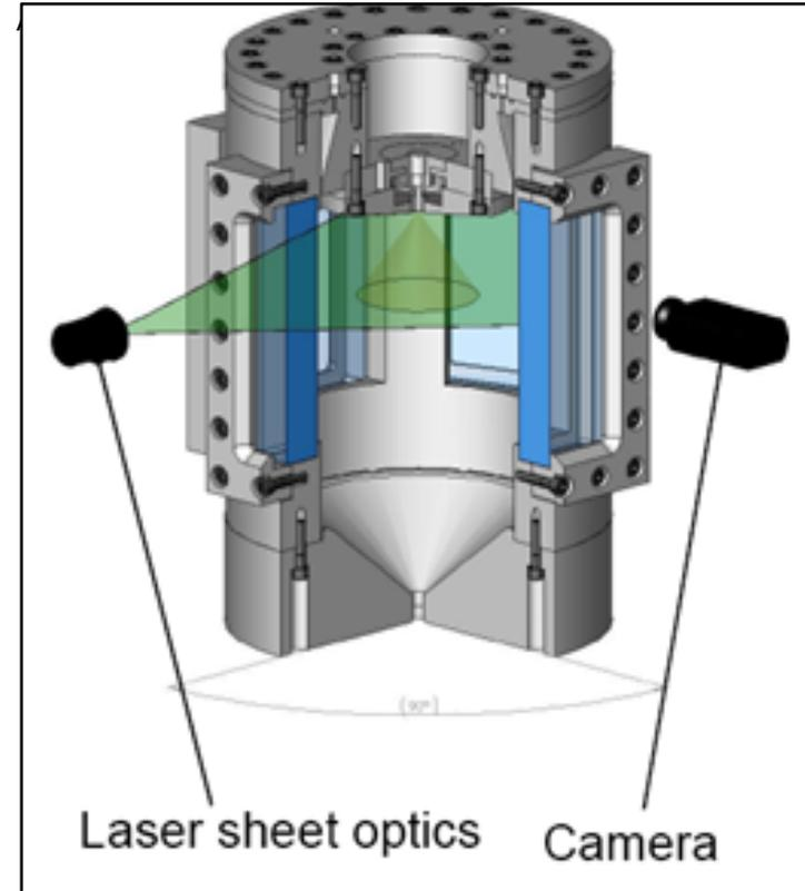
Pressurised Injector Test Chamber
