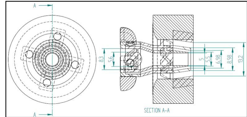
Prefilming Airblast Atomizer Prototype Design / Specification
