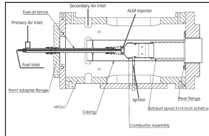
Schematic of RQL Burner in HPOC
