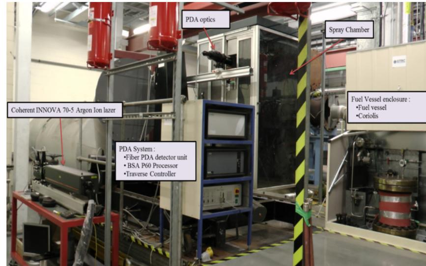
Large Scale Spray Chamber / Test Fuel Properties
