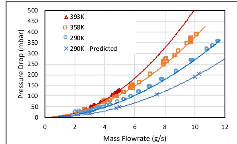
Pressure Drop vs Air Mass Flow
