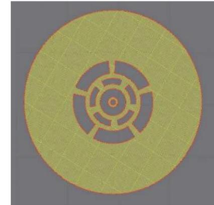
Injector Design with support structures, layer scan path
