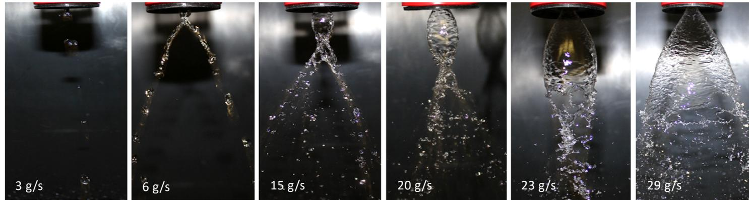
Development of spray in swirling pre-filming atomiser at increasing water mass flow rates
